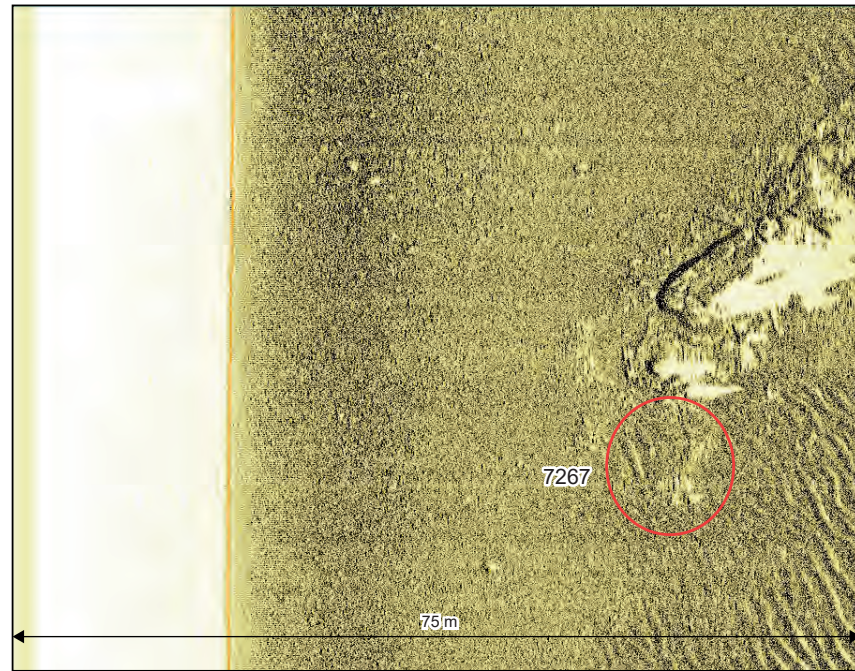
SSS waterfall image of seabed disturbance 7267 , measuring 9.6 x 7.8 x 0.5 m, looking north-west, 75 m range per channel
